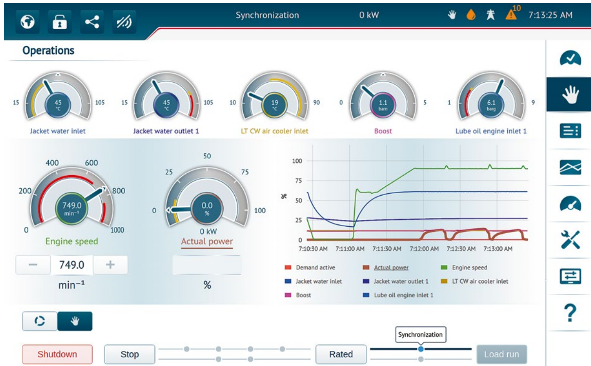
FIGURE 7 E 2 PILOT is a convenient multi-touch user interface for plant operators including trends, operation logs and test functions (© AVAT)
